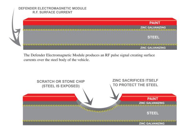
Zinc Galvanizing sacrifices itself to protect the steel and slow down the corrosion process.
