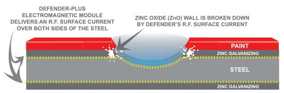
Once the steel is exposed, the surface currents produced from Defender-Plus Module start to breakdown the Zinc Oxide wall, allowing the Zinc Galvanizing to once again protect the steel surface and slowing down the corrosion process. In testing the corrosion rate was slowed by a factor of a 100 or up to a 99.7% reduction in corrosion.
