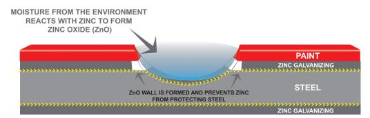
Zinc Galvanizing reacts to moisture in the environment causing Zinc Oxide (ZnO) to form. This renders the Zinc Galvanizing inert and unable to protect the steel, causing corrosion.
