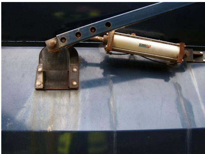
TWO-YEAR OLD DUMP BODY TARP ARM MOUNTING BRACKET AND CYLINDER
